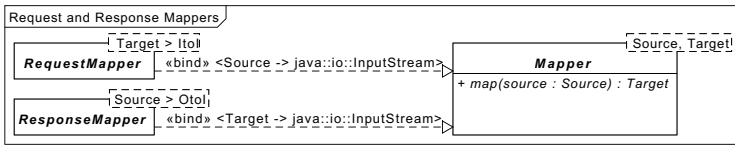
Fig. 3. The abstract Mapper class and its subclasses. Request mappers create inbound DTOs from input streams, whereas response mappers map outbound DTOs to technology-dependent client responses.
